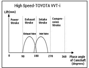
Fig1: lift vs phase angle diagram (toyota vvt-i)
